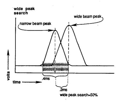
Figure 5. Graphic representation of ESP Dual-Beam Processor's wide peak search, which indicates how far on either side of the narrow peak echo to search for the wide peak echo of the same ping.
