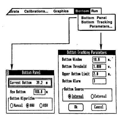
Figure 12. *Bottom* menu item of ESP Echo-Integrator, showing Bottom Panel and Bottom Tracking Parameters boxes.
