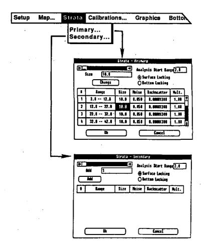
Figure 10. Strata menu item of ESP Echo-Integrator showing secondary strata which may be used to integrate the acoustic signal with a second set of parameters. Separate noise thresholds and backscattering cross sections may be applied to each of up to 200 strata.
