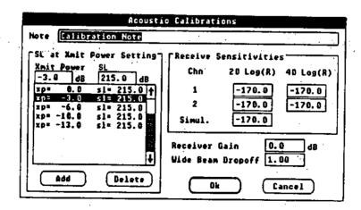
Figure 7. Acoustic Calibrations menu item of the ESP Dual-Beam Processor allows input of acoustic system's receiving sensitivities and source level measured at various transmit power settings.
