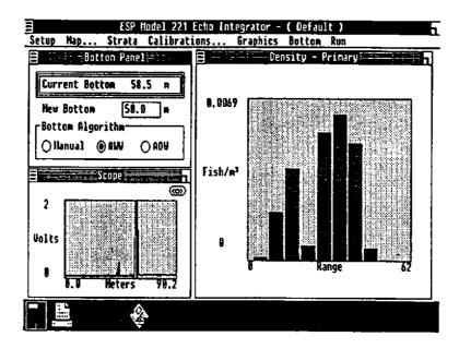
Figure 11. *Graphics* windows of ESP Echo-Integrator include real-time, on-screen displays of fish density histogram, bottom panel and oscilloscope.
