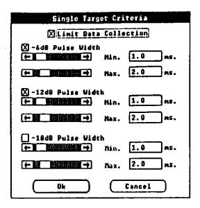
Figure 8. Single Target Criteria used by the ESP Dual-Beam Processor to classify echoes which exceed the noise threshold as either single or multiple targets.
