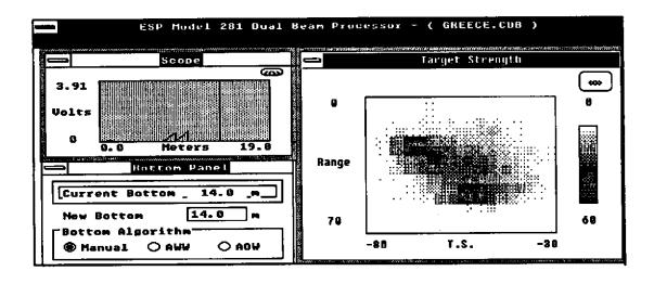
Figure 9. *Graphics* windows of ESP Dual-Beam Processor include real-time, on-screen displays of target strength histogram, bottom panel and oscilloscope.
