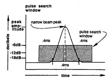
Figure 4. Graphic representation of pulse search window within which the ESP Dual-Beam processor searches for the -6 dB, -12 dB and -18 dB points of the narrow- and wide-beam echoes.
