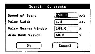
Figure 3. Sounding Constants menu item of ESP Dual-Beam Processor, showing dialog boxes for user input of processing parameters.
