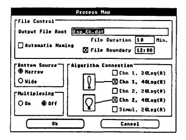
Figure 2. *Process Map* menu item of ESP Dual-Beam Processor, showing File Control, Bottom Source, Multiplexing and Algorithm Connection boxes.
