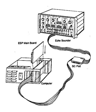
Figure 1. ESP computer and Signal Conditioning (SC) Pod connected to echo-sounder.
