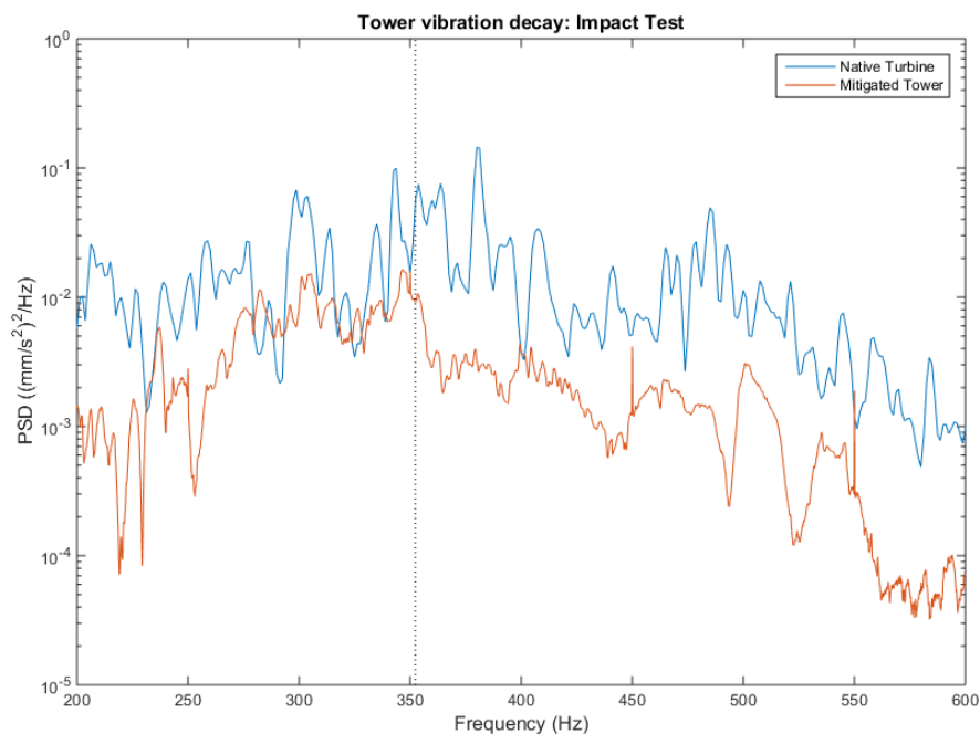
Figure 3: Power spectral density of the bottom of the native and mitigated tower after being excited by an impact hammer. The dotted line represents the problematic frequency for which the tower was damped.
