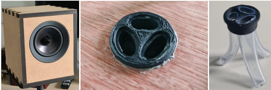
Figure 10 Prototype of 2L Satellite Loudspeaker with Branched Port Detail
