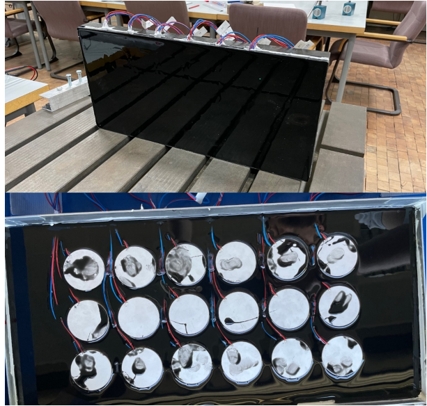
(b) GRP-plate with 3 x 6 piezoelectric actuators during (bottom) and after the potting compound is attached (top)
