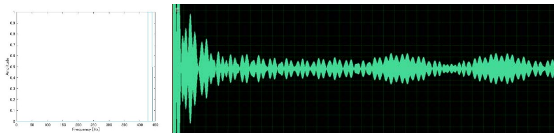
Figure 13. In-phase sinusoidal spikes with the common tolerance frequency of 0.1Hz between frequency area of 440 and 426.25 Hz. Note that the distribution of frequencies here gives not pitch divergence but rhythmic ones.
