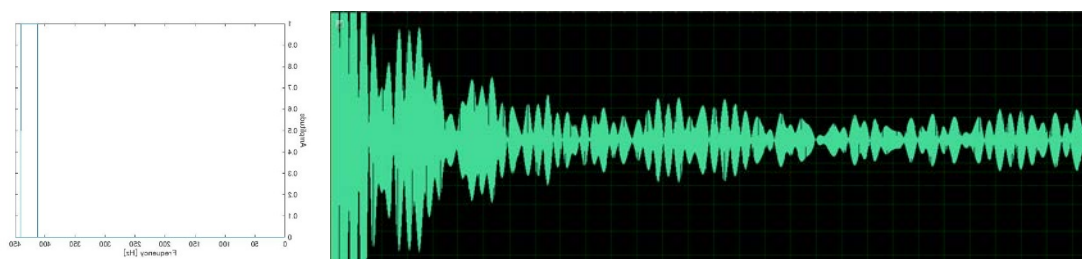
Figure 14. In-phase sinusoidal spikes with the common tolerance frequency of 0.1Hz between frequency area of 440 and 412.5 Hz. The sound quality begins differ from that of single sinusoid; a cognitive phenomenon caused by human inner ears and central cognitive system.
