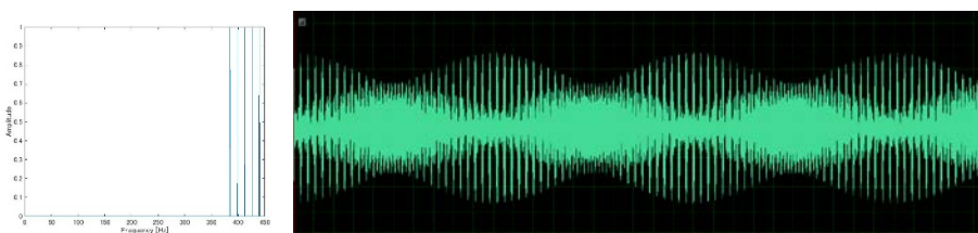
Figure 10. 5 Bright lines' spectral spikes and superposed sinusoidal wave form (440Hz、412.5Hz and 385Hz). The non-linearity of subjective sound image increases more.
