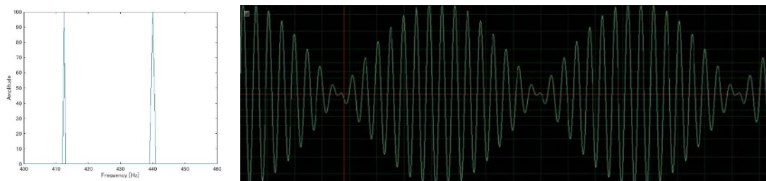
Figure 6. 2 Bright lines' spectral spikes and superposed sinusoidal wave form(440Hz, 412.5Hz)
