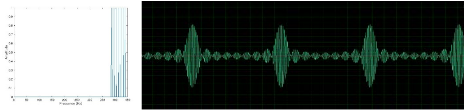
Figure 11. above 9 (above)/ 17(beneath) Bright lines' spectral spikes and superposed sinusoidal wave form (evenly divided between 440Hz and 385Hz). As the result of phase matching we hear interfering attacks with the frequency of common tolerance.
