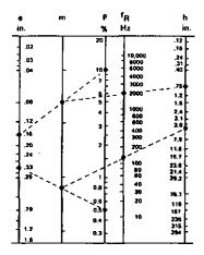
EXAMPLE A: TO CALCULATE THE RESONANCE FREQUENCY OF A GIVEN TUNED SOUND ABSORBER.
