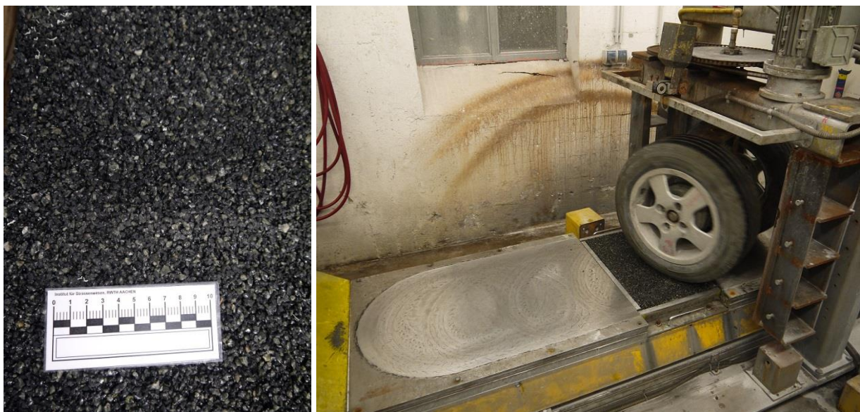
Figure 6 Test slab of the first NEREiDE PERS mix (left hand side) and testing on the ARTe (the result was not yet satisfactory)
