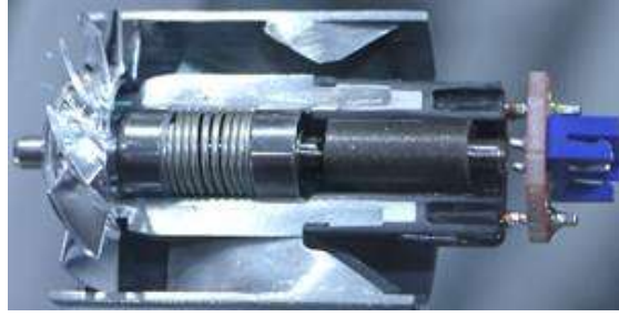
Figure 4: Main structure of the high-speed brushless motor.
