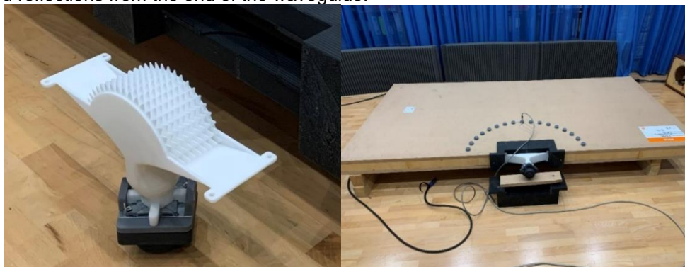
Figure 11: Measurement set up photos. Left: 3D printed optimised wave-shaper and horn, Right: Measurement waveguide with microphone positioned on axis
