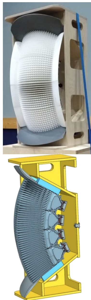
Figure 13: 60^\circ \times 120^\circ Source with 4 1-inch compression drivers. Top: photo, Bottom: CAD section view
