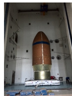
Figure 8: Test acoustic chamber and payload fairing
