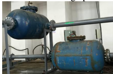
Figure 3: Water mufflers used in the experiment
