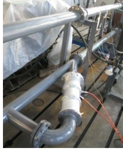
Figure 4: Underwater acoustic transducer used in the experiment
