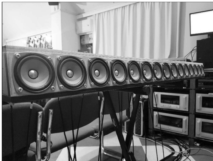
Figure 4: A photograph of the 3-channel, 6-way OPSODIS sound bar used for the purpose of this paper.
