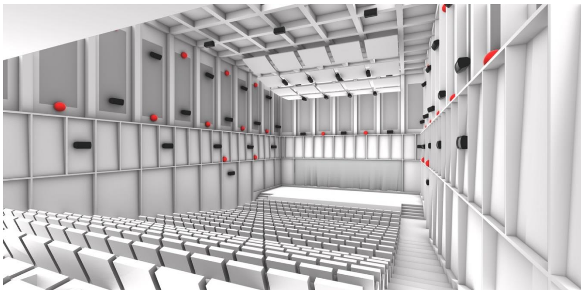
Figure 10. Interior view of the acoustic model showing the distribution of loudspeakers and microphones of the active acoustic system.
