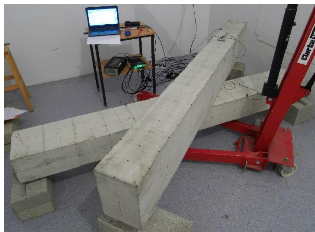
Figure 1 - Test setup showing the test equipment and the X-shape junction formed by beams 1 and 2.
