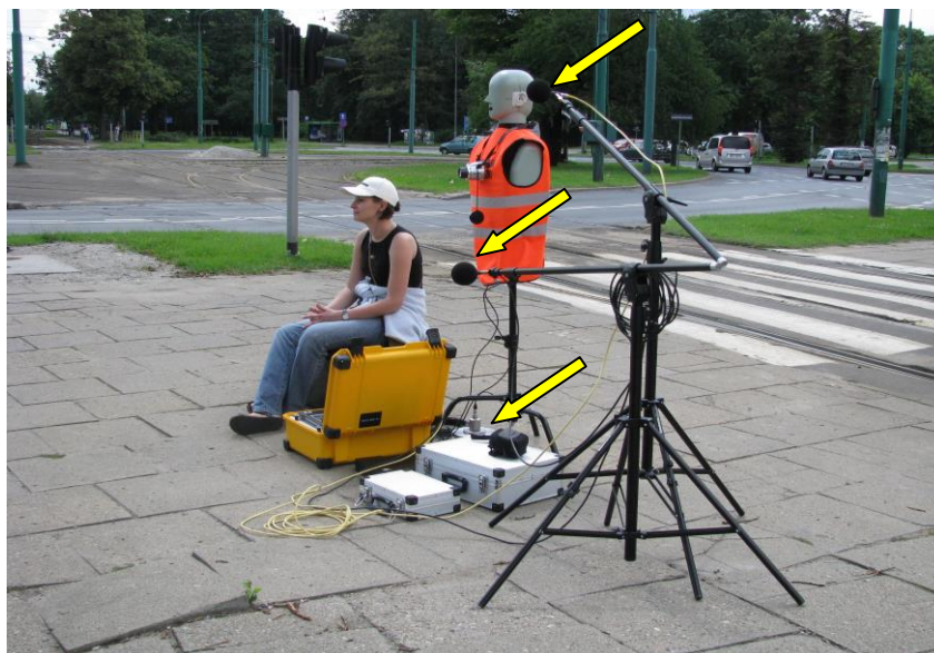
Figure 10: Time variations of noise level at the heights of 90 and 160 cm at the tram stop (microphones set perpendicularly to the direction of tram motion).
