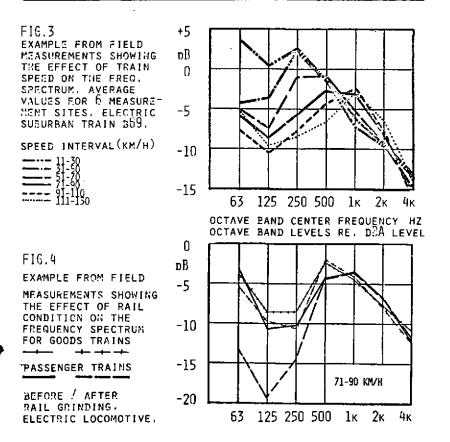
MEASUREMENT POSITION 7.5M FROM TRACK CENTER LINE 2M AROVE RAIL LEVEL. ENERGY EQUIVALENT LEVELS CORRECTED TO A TRAIN LENGTH OF 100M (SEE REF.3).
