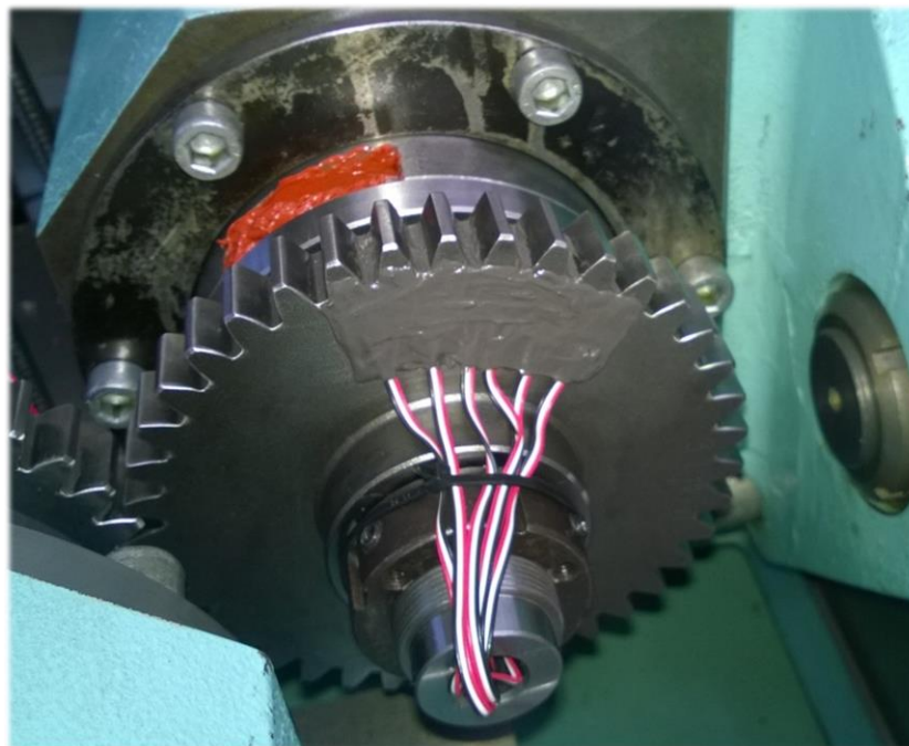
Figure 9: Strain gauge details of gears connections.
