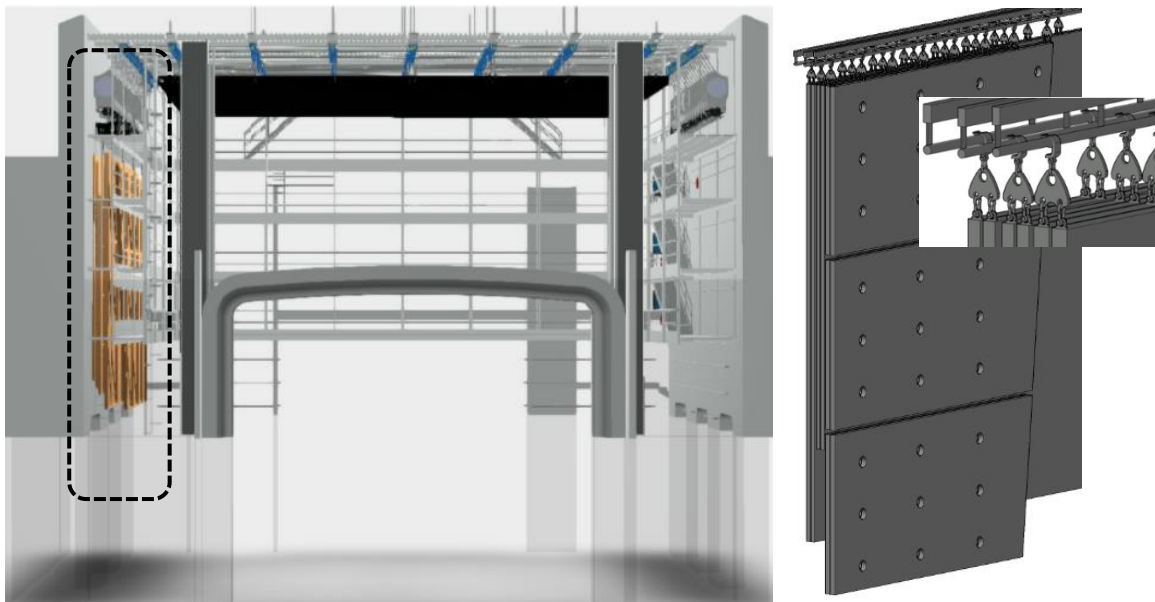
Figure 2. Stage general front view and stored acoustic shell detail (folded)
