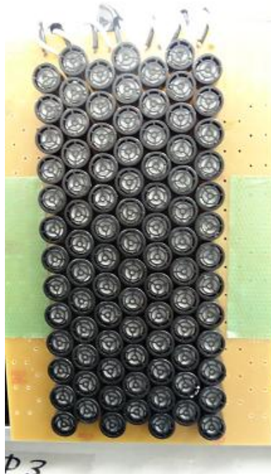
Figure 3: 7ch parametric loudspeaker.
