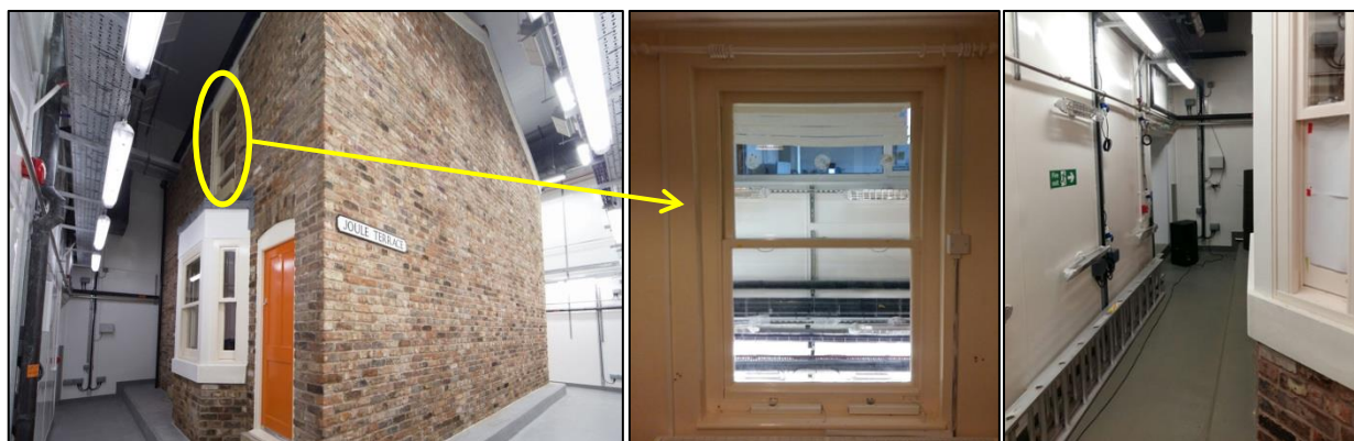
Figure 1: the energy house (left), the window tested (centre) and the loudspeaker in the house compound (right)
