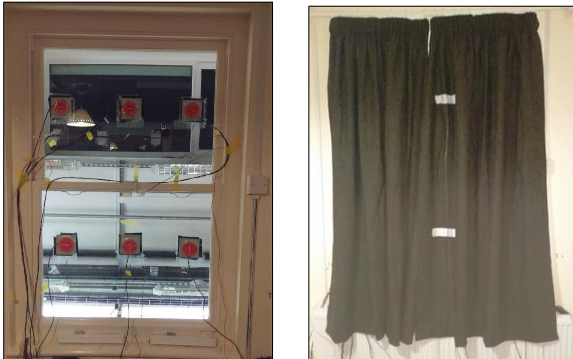
Figure 2: U-value measurement setup showing position of heat flux sensors (left) and with tweed curtain (right)
