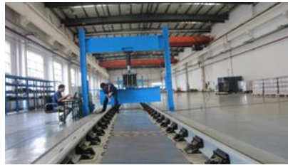
Figure 6: laboratory 1:1 simulation track system.
