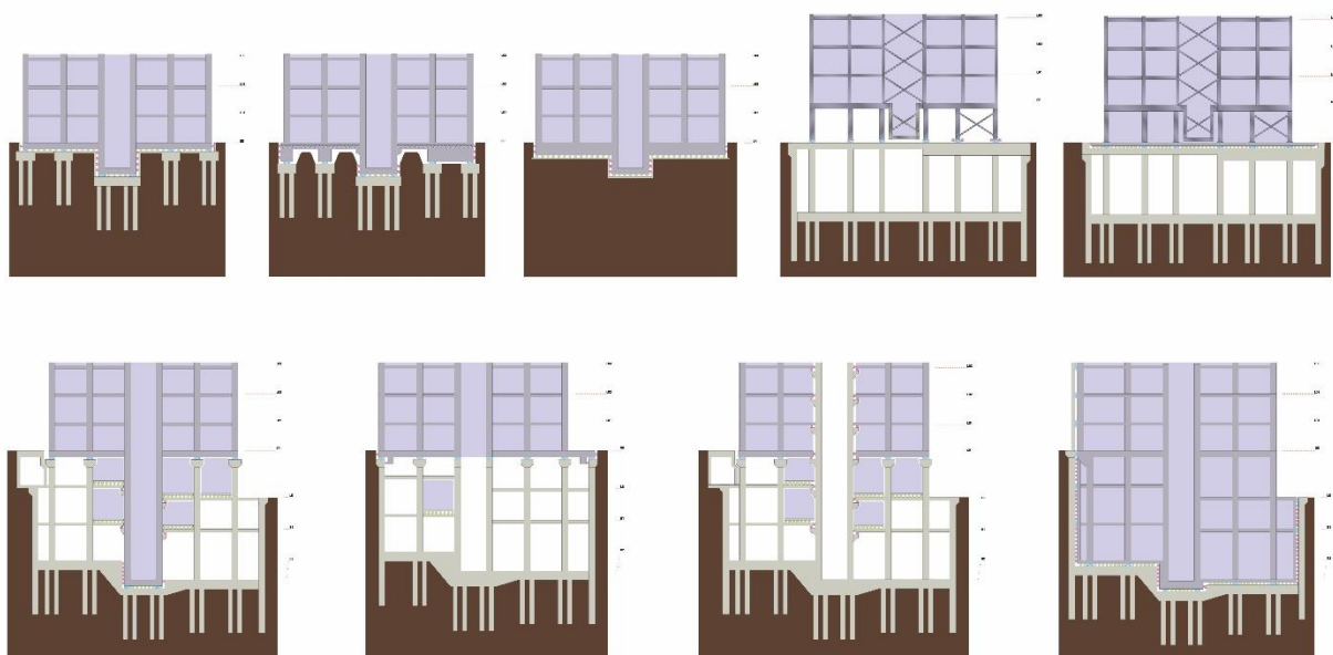
Figure 1: Examples of vibration isolated building design schemes showing the variety of foundation and super-structure designs
