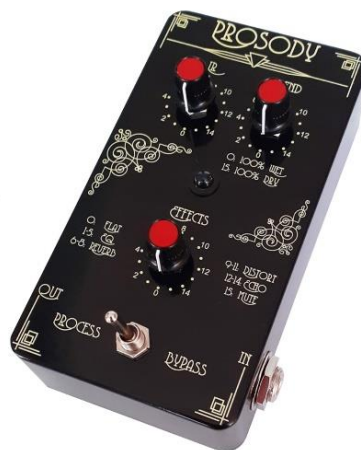
Figure 5. The Prosody pedal, which performs real-time convolution of an acoustic instrument impulse response with a signal from its electric equivalent.
