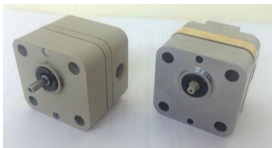
Figure 1: Physical configuration of the micropump made of different materials.
