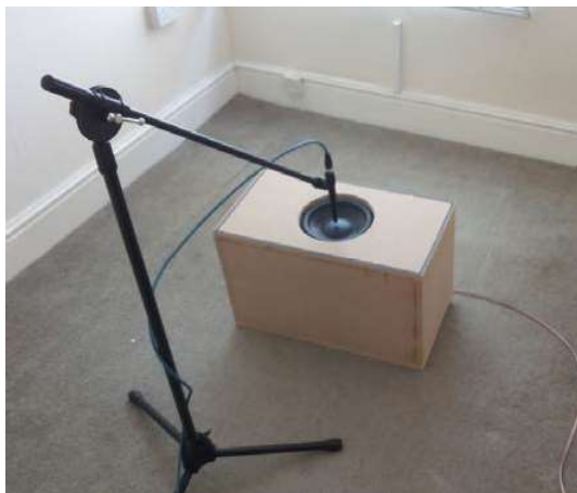
Figure 16 : near field measurement setup
