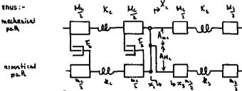
Dashpots,  $\frac{r}{2}$ , are included to account for the flow resistivity of air through the foam, this constituting the second coupling effect between the accoustic and mechanical systems.
