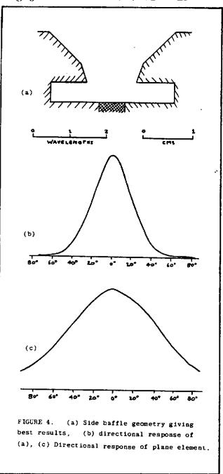
3 dB beamwidth is  $30^{\circ}$ . Since the Fourier transform of a
