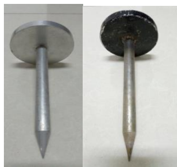
(a) Aluminium-made Mount (b) Iron-made mount Figure 3 Pictures of Mounts
