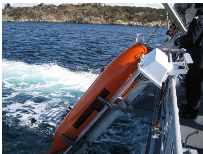
Fig. 1. HUGIN 1000-MR AUV with HISAS 1030 during recovery on the Royal Norwegian Navy mine hunter Hinnøy.
