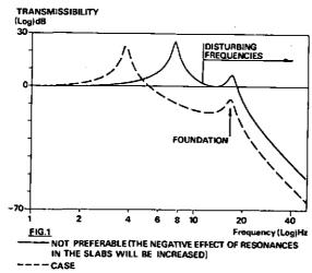
In this project the first thing to check in practice was the natural frequencies of the concrete slabs. By means of impact excitations and an optic x-y writer approximately 15 Hz was registered in most cases.
