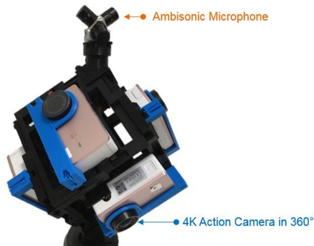
Figure 1: Omnidirectional video recording setup with 4K cameras and Ambisonic microphone
