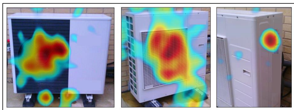
Figure 3 Acoustic camera images of air source heat pumps
