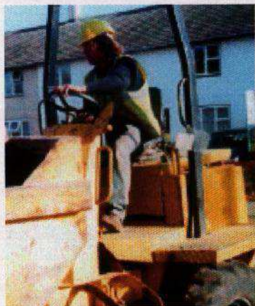
A typical source of whole body vibration applied to the feet and the seat – a dump truck cab
