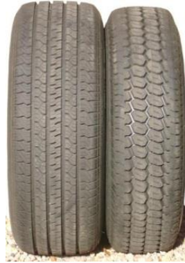
Figure 1: Picture of the two standard tyres used for CPX-measurements. Left: SRTT (P1), right: Avon AV4 (H1).
