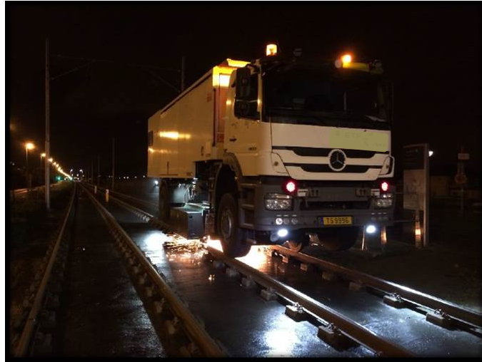
Figure 1: Rail grinder on traditional slab track – December 2016.
