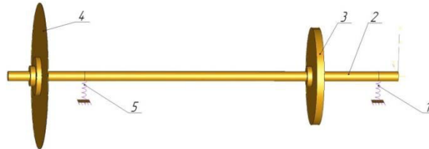
Figure 7: Numerical rotor system model: 1,5 - rotor supports, 2 - rotor shaft, 3 - load disk (superelement), 4 - flexible disk (superelement)
