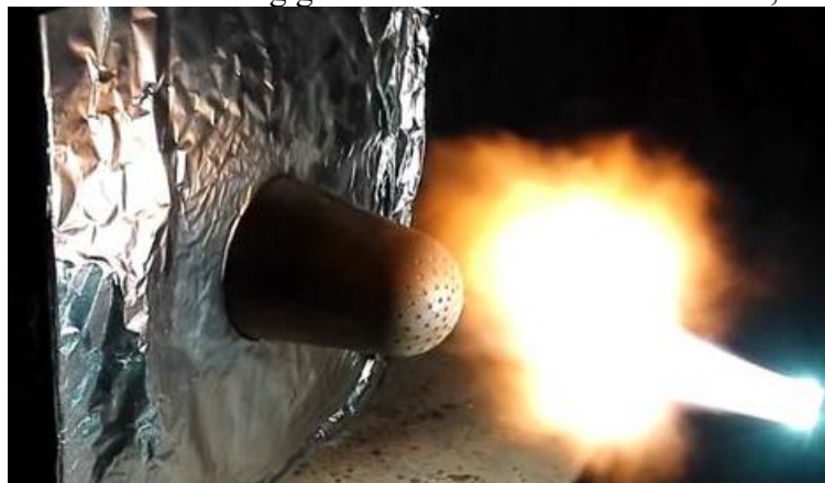
Figure 16: Cone heated by welding gun (with active cooling)
