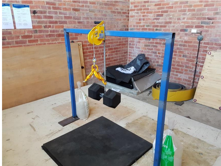
Figure 1: Weight rack with hand winch used to produce repeatable tests
