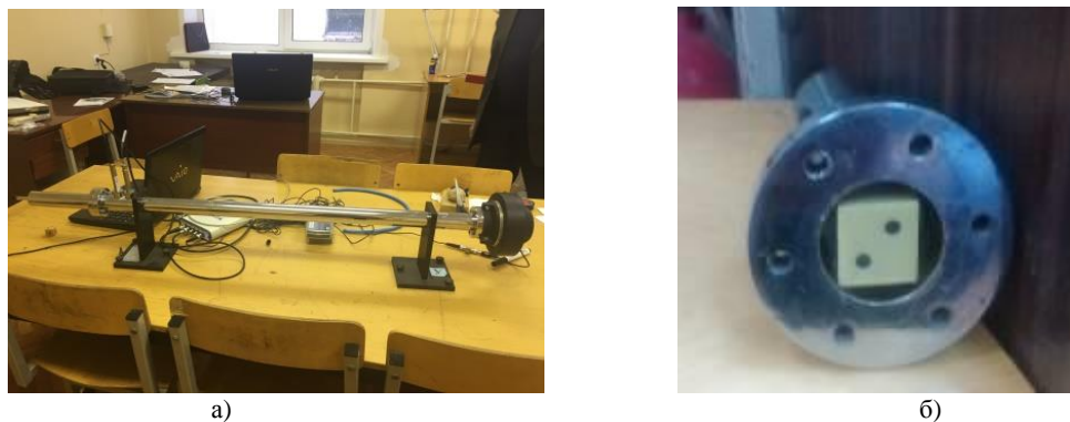
Figure 1: The impedance tube (a) and the sample in the form of Helmholtz resonator (b).
