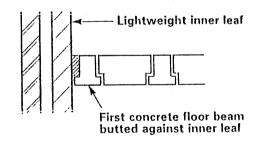
B. as for A, with one row of dense concrete blocks replacing the lighter density blocks in the inner leaf at the level of the separating floor;
