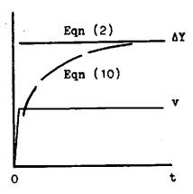
Now consider a reference motion on which is superposed a constant acceleration in sway  $\dot{\mathbf{v}}_{o}$ , which develops rapidly at time  $\mathbf{t}=\mathbf{o}$ .
