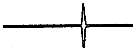
FIGURE 6 PULSE ARRIVAL A 1 msec PARAMETRIC PULSE AT 15 kHz RECEIVED AT A RANGE OF 412 yd
