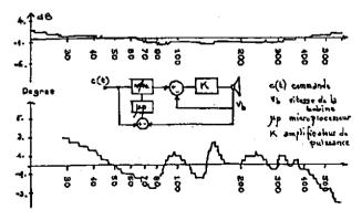
The output signal is the velocity of the driver coil. In fact the velocity of the membrane must be controlled. It is not easy to avoid the convolution between these two velocities. § 3 shows how a new technique replacing the analog network in front of the loop is more suitable. An alternative method is to control other sources such as acoustic drivers [3].
