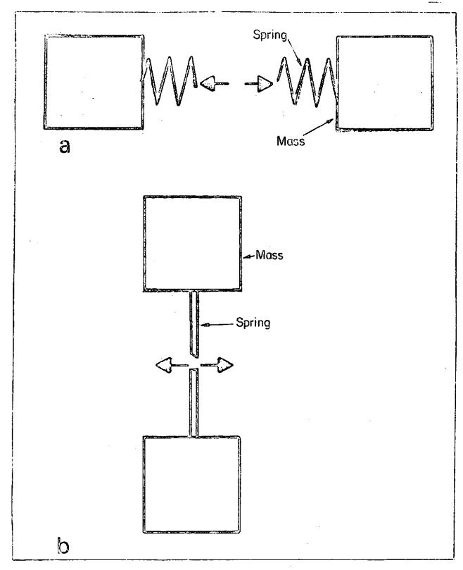
Fig. 3 Diagrams of 'lumped' mechanical resonant systems;-
