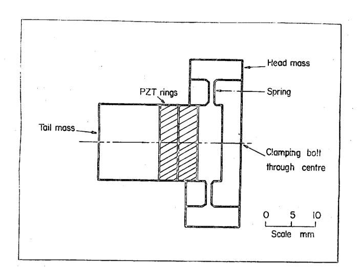
Fig. 4 'Flywheel' transducer configuration, drawn to scale.
