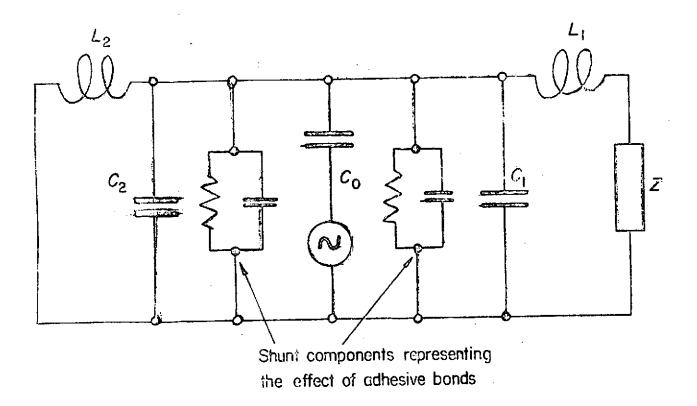
Fig. 2 Electrical analogue circuit of 'sandwich' type transducer.
