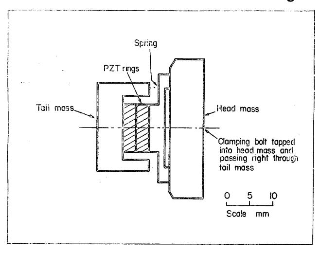
Fig. 5 Modified 'sandwich' type, incorporating additional flexural spring, drawn to scale. Aluminium head; brass tail; frequency 10 kHz.
