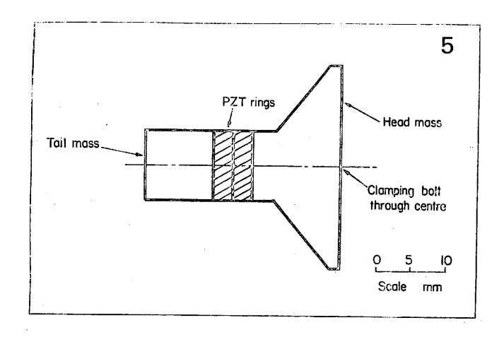
Fig. 1 'Sandwich' type transducer (general configuration, drawn to scale). Aluminium head; brass tail; frequency 25 kHz.
