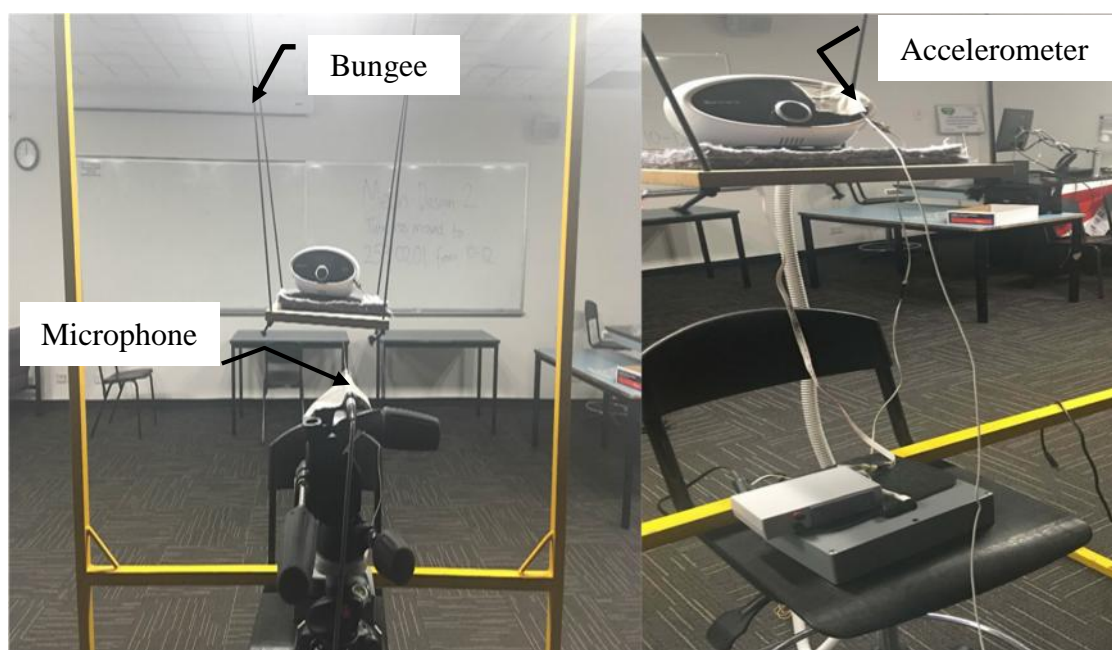
Figure 2: Experiment set up for CPAP device
