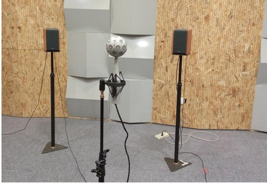
Figure 1: Eigenmike microphone and two sound sources.
