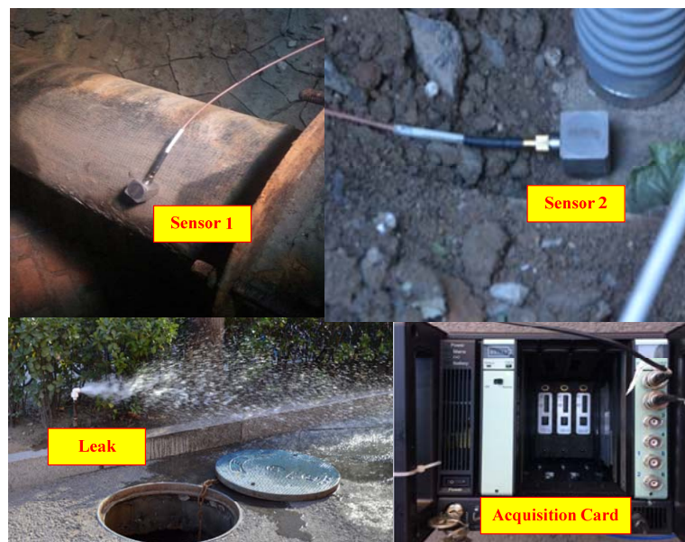
Figure 3: Test rig in the field.
