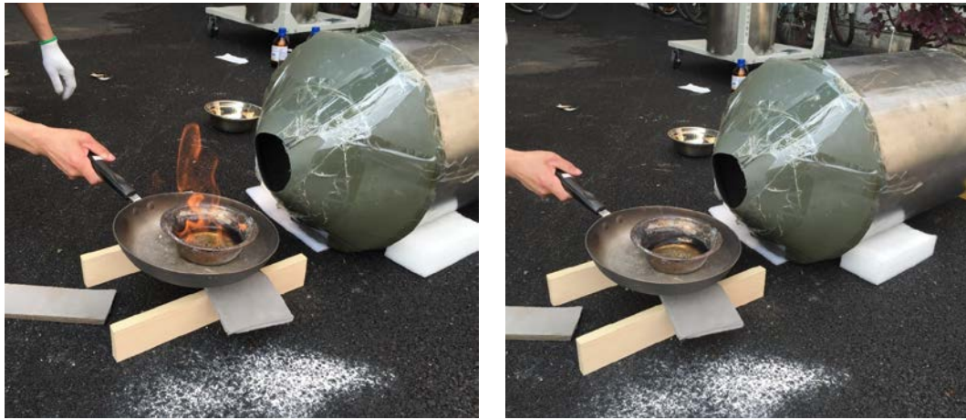
Fig. 5. Experimental test. Left: the fire flame before the acoustic suppression. Right: fire extinction after the acoustic suppression.
