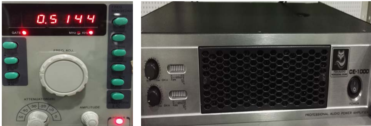
Fig. 2. Signal generator and power amplifier. Left: signal generator. Right: power amplifier
