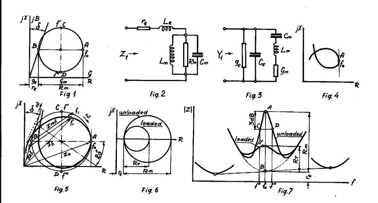
loop may be found when the phasors of the electrical and mechanical branch are added for corresponding frequencies. This is shown on fig.5 using only the impedance terms for simplicity. The loop is "pulled" inside the motional circle and its distortion depends on frequency scale along the electrical line, i.e. on the  $L_{\rm c}$  and  $R_{\rm m}$  values (or coupling coefficient k).
