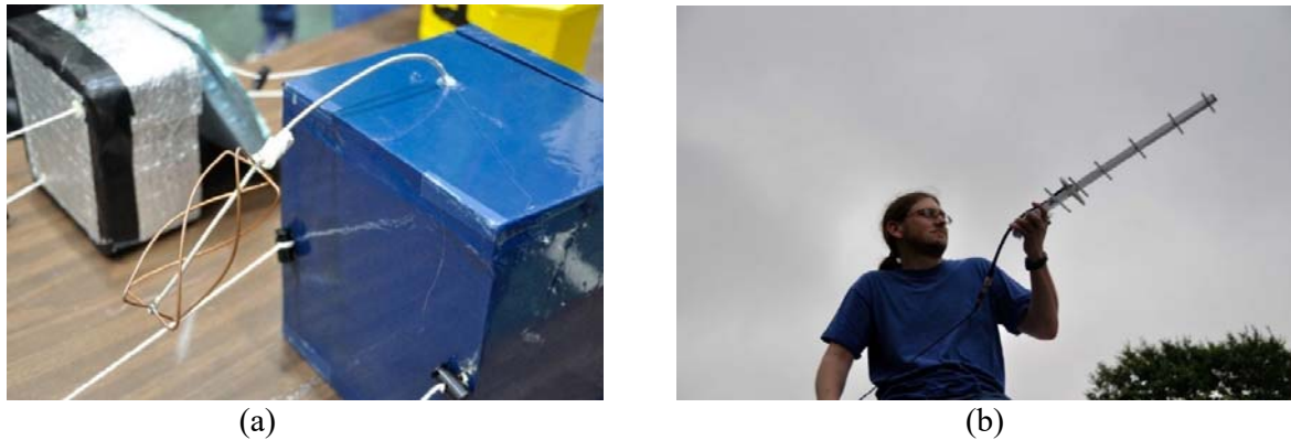
Figure 5. (a) payload on strings before launch, (b) hand-held receiving Yagi antenna.
